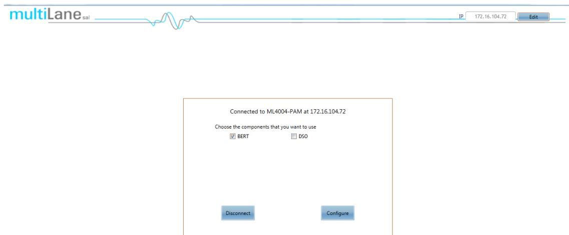
When you enter the IP address and connect to the instrument, you are presented with the above menu. Choose if you plan on using the ML4004-PAM as BERT only, Scope only or both.
