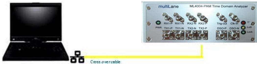
Figure 33: ML4004-PAM connected with Ethernet crossover cable
